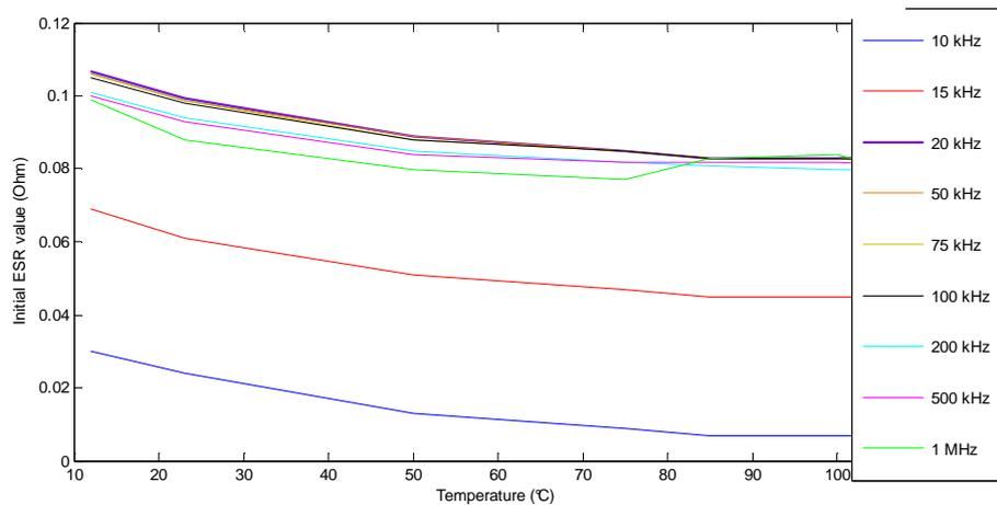
**Figure B2. Experimental curve describing the variation of the initial ESR value  $ESR_0(T^{me})$ , in Ohm, at different measurement frequencies**
