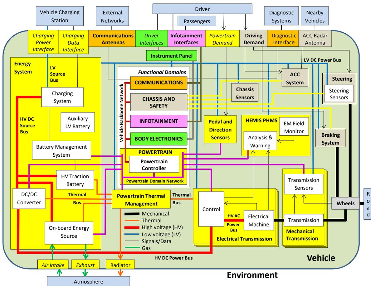
Figure 4: HEMIS generic electric vehicle architecture - Functional view
