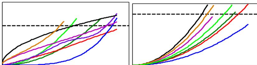
Figure 3: Example of a signal characterized by bad trendability (left) and a signal characterized by good trendability (right)
