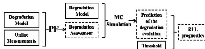
Figure B1. Sketch of the PF approach to fault prognostics
